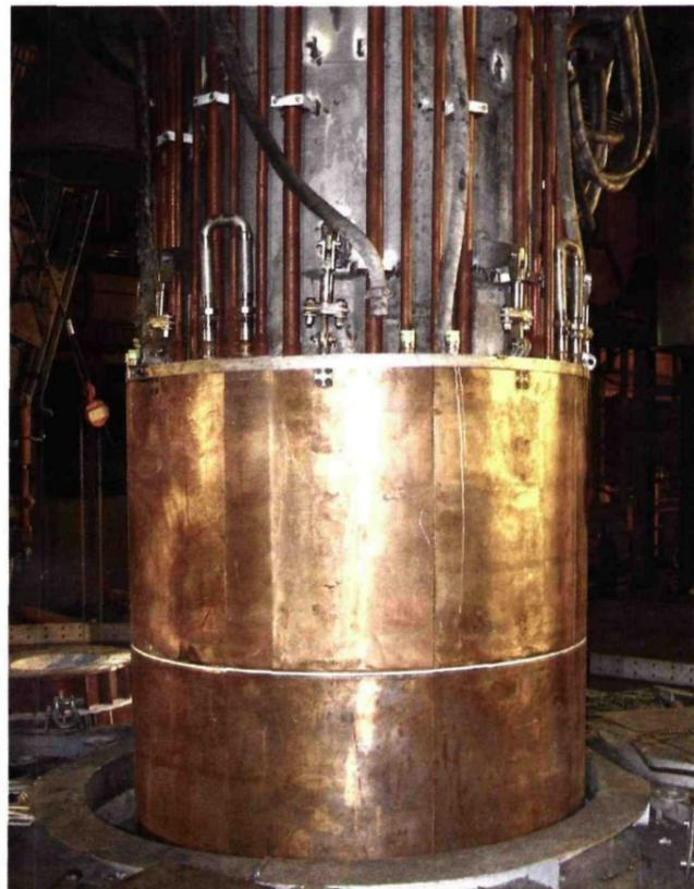
With the taller pressure rings, the insulation between the shields and pressure rings will never be exposed to the heat in the furnace.
