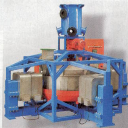
HIGH INTENSITY One of the magnetic separators supplied by Multotec Magnetics to a customer in India
